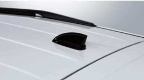
Shark-fin antenna with glonass, DAB and GSM
