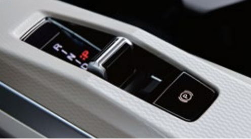
Electronic parking brake with auto-hold function
