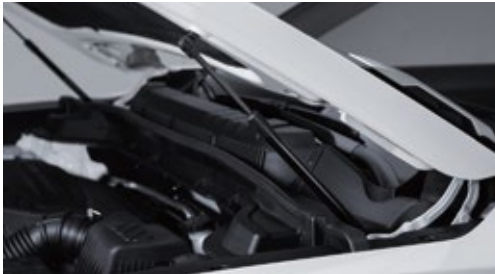
Gas strut bonnet supports
